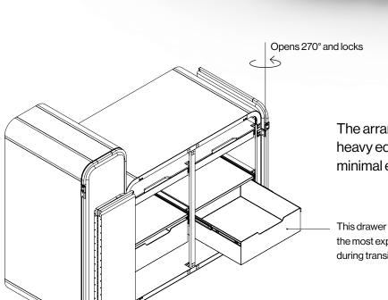
The arrangement of drawers allows heavy equipment to be lifted with minimal effort.
